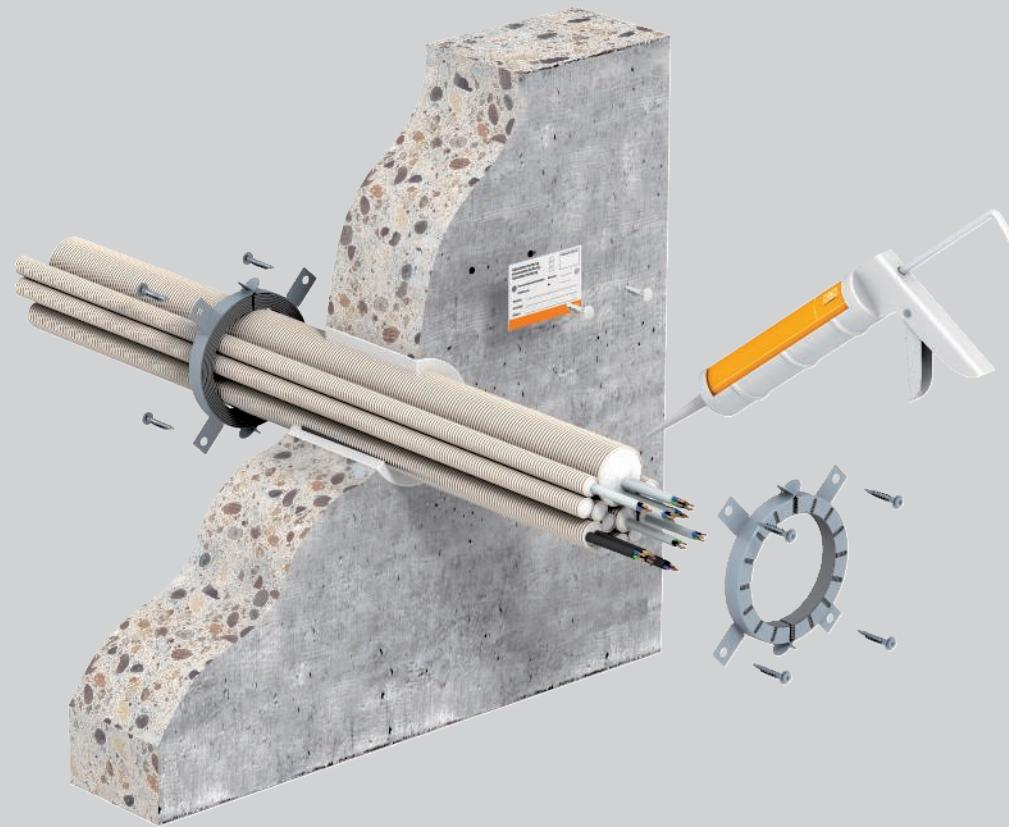
The PYROCOMB® Tubes system is used to create cable insulation with pipe sleeves. The system comprises multiple sizes of the pipe sleeve, type TCX. This allows simple insulation of bundles of plastic electrical installation pipes, rigid or flexible, up to a size of M63. It is irrelevant whether the pipes are filled with cables
