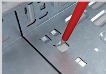
Bending the locking straps in the base.
