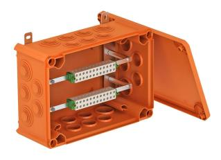
Halogen-free junction box as small data distributor with pre-mounted, soft plug-in seals, approved for the maintenance of electrical functionality according to DIN 4102 Part 12. Maintenance of electrical functionality classes E30 to E90
