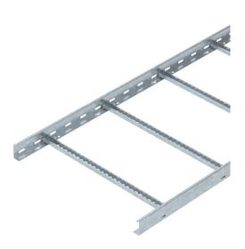
Cable ladder with a 60 mm side height with welded C30 profile rungs which are open in an upwards direction. Rolled side rail for reinforcement and as edge protection. Fastening to the bracket takes place using hold-down clamps, type LKS 40. The slot dimension of the rung is 16.5 mm and the appropriate clamp clip is type BS-H....
