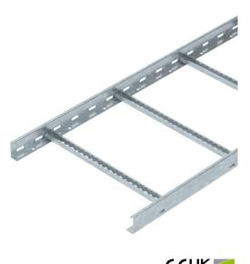
Cable ladder with a 60 mm side height with welded C30 profile rungs which are open in an upwards direction. Rolled side rail for reinforcement and as edge protection. Fastening to the bracket takes place using hold-down clamps, type LKS 40. The slot dimension of the rung is 16.5 mm and the appropriate clamp clip is type BS-H....
