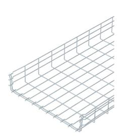
Mesh cable tray with shaped connector of side height 105 mm. No additional connection components are required for the mesh cable tray, it is simply interlocked. The grid width is 50 x 100 mm. Magnetic shield insulation without cover 15 dB, with cover 25 dB.
