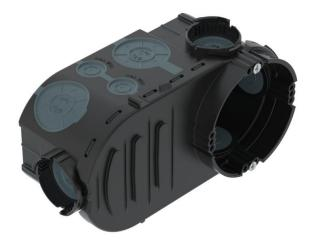
Flush-mounted electronics box, with additional clamping space and airtight membrane entries, for use in masonry with an installation depth of at least 67 mm.
