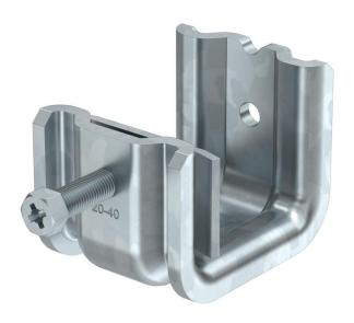
This type of support clamp is pushed onto the support and fixed to the girder or flat iron using a pressure trough and bolt (M8). The hexagonal bolt has a WAF of 10 mm. In the clip element also two more M8 threads are introduced, for example to attach threaded rods.
