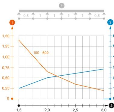
Load diagram, cable ladder, type SLZ ALU
