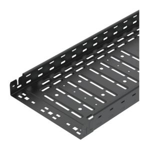
Cable tray with integrated quick-fastening system. Strip-galvanised surface, visible areas powder-coated in jet black (RAL 9005). Continuous side perforations of 7  $\times$  20 mm for the installation of additional connection and mounting components. With 11 mm perforation in the base for direct threaded rod suspension. Usable length 3,000 mm.
