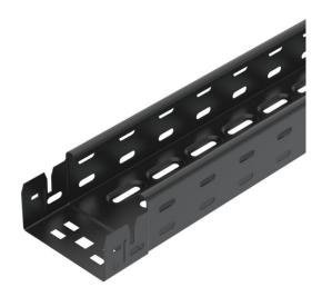
Cable tray with integrated quick-fastening system. Strip-galvanised surface, visible areas powder-coated in jet black (RAL 9005). Continuous side perforations of 7  $\times$  20 mm for the installation of additional connection and mounting components. With 11 mm perforation in the base for direct threaded rod suspension. Usable length 3,000 mm.
