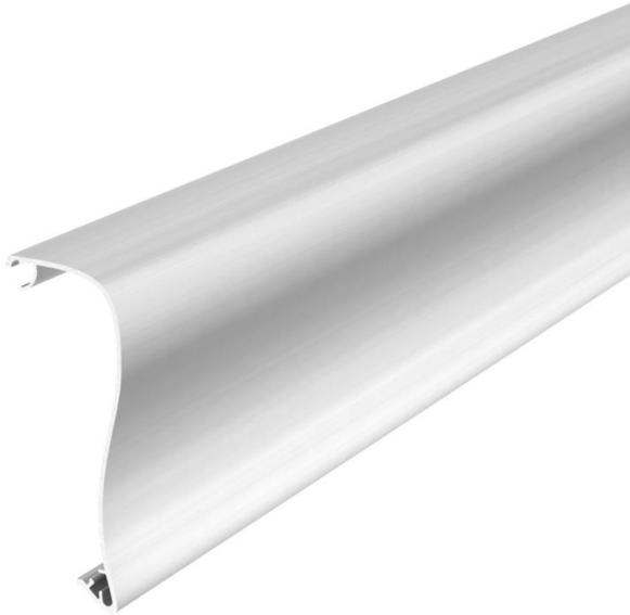
Trunking cover to create a design device installation trunking of the GAD series. "Swing" design version for complete coverage of the system opening and the switching and plug-in devices. The GAD OTA cover adapters are essential and must be planned on the trunking section with a max. spacing of 50 cm. A GAD OTD spacer must be placed between the trunking covers. Standard version in anodised aluminium, different decoration on request.
