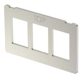
Support plate to accept three data connection modules of the following types: AMP TYCO: SL series 110Connect and Toolless, AMP-Twist; Brand-Rex: unshielded; GG45; TKM RJ MOD; Nexans: LANmark with Adapter Clip. Dimensions of a mounting opening in mm: 20.10 x 14.80.
