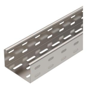
MKS 60 = Medium-duty cable tray system with a side height of 60 mm. Connecting parts should be ordered in the appropriate quantity. Magnetic shield insulation without cover 20 dB, with cover 50 dB.
