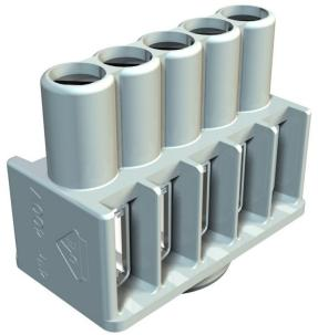
Terminals and screws made of steel, galvanised and transparent-chromated, nominal cross-section 1  $\div$  4 mm², rated voltage 400 V, five-pole, with socket terminals, max. connectable cross-sections per terminal: 4x2.5 mm², 5x1.5 mm² or
