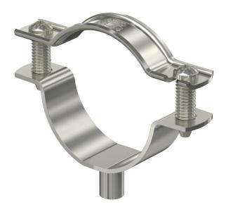
Spacer clip for the installation of pipes and cables on walls, ceiling and floors. With self-locking upper part. Surfaces G and FT from a clip size of 20 are suitable for installation with a nail device or a bolt-firing tool.
