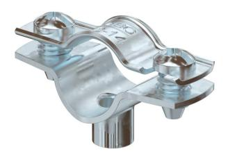
Spacer clip for the installation of pipes and cables on walls, ceiling and floors. With self-locking upper part. Surfaces G and FT from a clip size of 20 are suitable for installation with a nail device or a bolt-firing tool.
