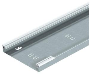
On-floor trunking base, 1 compartment, for blank/mounting lid with slope on one side, with plug-fit aluminium side profiles for layering and fixing the trunking lid, metal floor base with holding shackles for max. two plug-in, self-contacting dividers and groove for earth conductor clamp. Trunking height suitable for installation of Telitanks or service outlets of nominal size 4, 6, 9.
